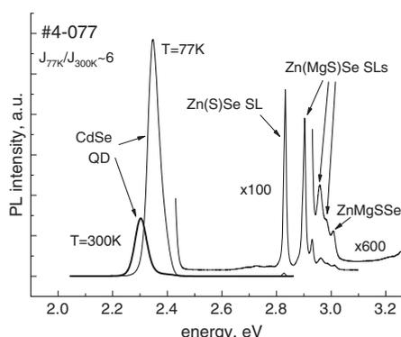
**Fig. 2** Surface PL spectra of Cd(Zn)Se/ZnMgSSe QD GIW laser heterostructure at 77 and 300 K
