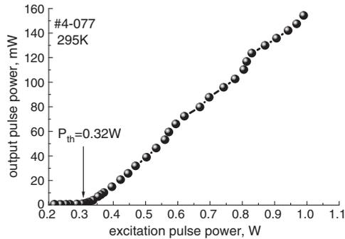
**Fig. 3** Cd(Zn)Se/ZnMgSSe GIW QD laser output against excitation power supplied by blue-violet InGaN/GaN LD ( $\lambda_{\text{exc}} = 416 \text{ nm}$ ,  $\tau = 50 \text{ ns}$ ,  $f = 1 \text{ kHz}$ )
