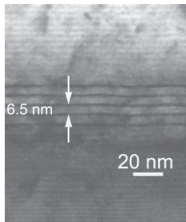
**Fig. 1** Bright field cross-section TEM image of Cd(Zn)Se/ZnMgSSe QD laser heterostructure with GIW waveguide and five QD sheets in active region
